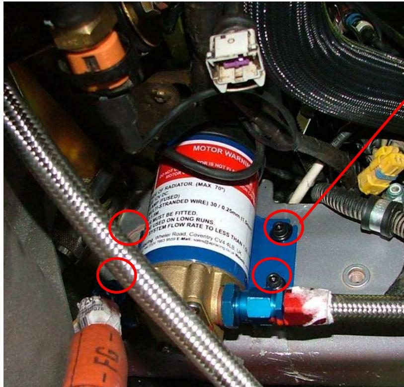
**Fit the oil pump on the left chassis frame, with 4 « Rivkle » dia 6mm.**
